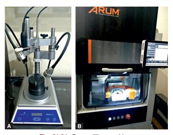
Fig. 21.21: Copy milling machines
