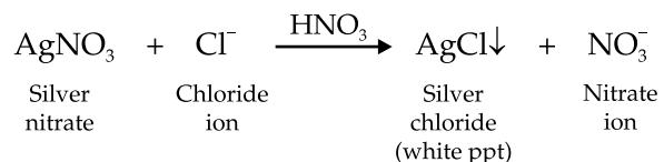
The opalescence obtained with sample is compared with standard opalescence produced from a definite quantity of chloride ions in the form of sodium chloride. Both the cylinders are viewed transversely against a dark background.
