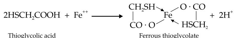
This ferrous thioglycolate formed is colourless in acidic medium but in alkaline medium it gives purple colour. Citric acid prevents precipitation of iron with ammonia and keeps iron in solution by forming a soluble complex with iron.
