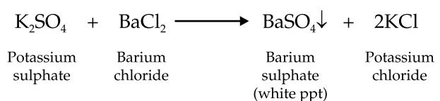
The barium sulphate, prepared *in situ*, assists rapid and complete precipitation by seeding. Test solution contains a small amount of potassium sulphate to increase the sensitivity of the test. Sulphate ion impurity in the sample will produce barium sulphate in excess of already dissolved amount and produce turbidity. Small amount of ethanol is added to prevent supersaturation of barium sulphate. Acetic acid is used as acidifying agent.
