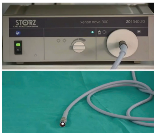
Fig. 7.7: Light source and light cables
