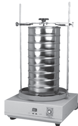
Fig. 1.1: Sieve shaker (grain size analysis) (Courtesy: AIMIL Ltd.)
