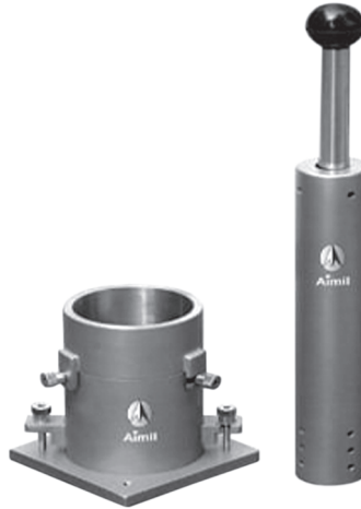
Fig. 5.1: Shows the apparatus for compaction test (Courtesy: AIMIL Ltd.)
