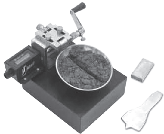
Fig. 2.1: Liquid limit test apparatus (Courtesy: AIMIL Ltd.)
