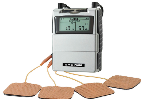
Fig. 3.1: Electric nerve muscle stimulator (Pocket size)
