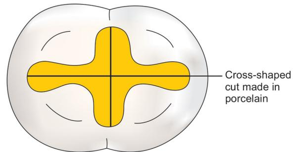
**Fig. 21.11:** Crosscutting method for reducing shrinkage in porcelain
