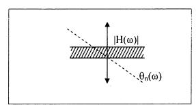
For Distortion Less filter  $Y(j\omega) = A(j\omega) \cdot X(j\omega)$   $H(j\omega) = A e^{-j\omega}$ Magnitude  $\rightarrow$  constant Phase  $\rightarrow$  linear
