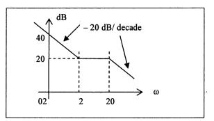
Since at  $\omega = 2$  rad/sec, slope changes from -20 dB/ decade, then there would be zero at  $\omega = 2$
