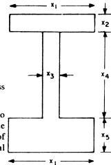
Considering next the shearing stresses, codes often prescribe a maximum average shearing stress, and a peak shearing stress, max, neither of which may be exceeded in the beam.
