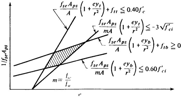
Fig. 7-5 Graphical solution of four equations in solving for the prestressing force and eccentricity.
