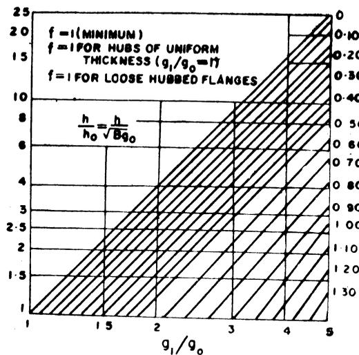
Fig. 7.9 Values of  $f$  (hub stress correction factor)
